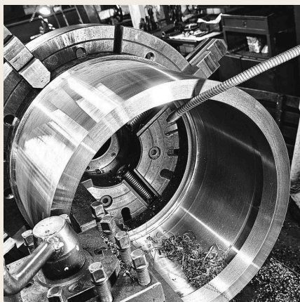
TURNING ON A FOUR-JAW CHUCK
