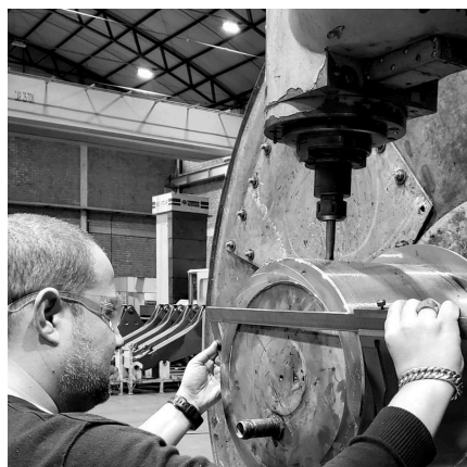
DIMENSIONAL INSPECTION ON THE MACHINE
