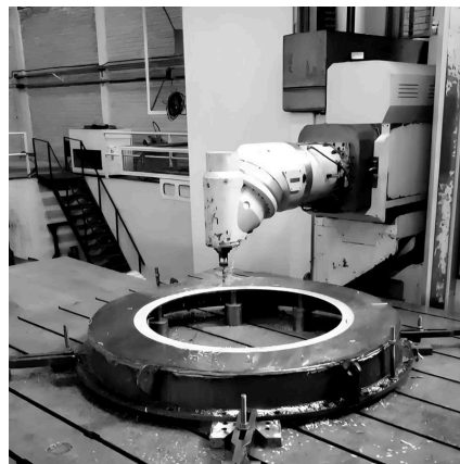
LARGE-DIAMETER RING BEING MILLED
