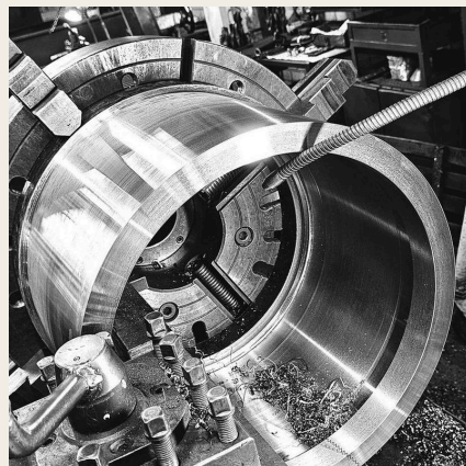
BUSHING TURNING · CONTINUOUS CHIP
