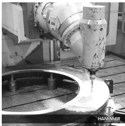
RING MACHINED ON A CNC BORING MILL
