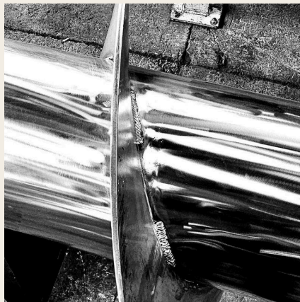
FLIGHT WELDED TO THE CENTRE PIPE
